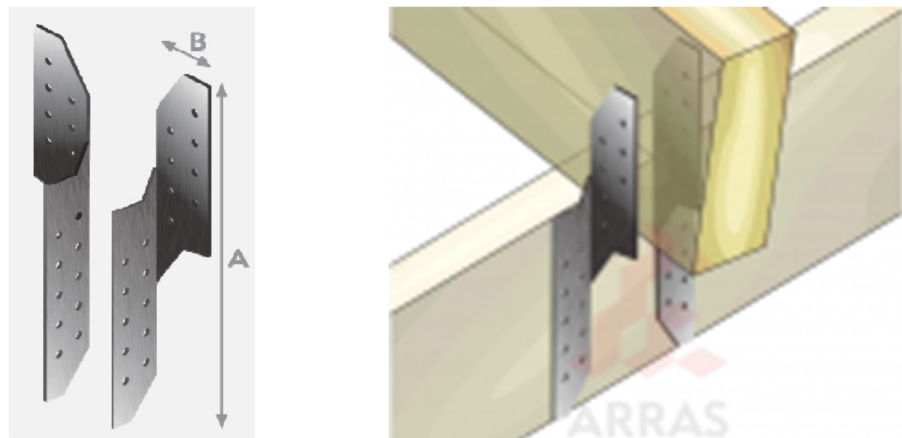
Figure 1. Types of right and left hand purlin anchors and the typical use of connectors.
